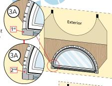
B. **Apply side flashing tape.** Cut two pieces of flashing tape 4" longer than the frame height of the window. Apply one piece 1/2" up onto the frame cladding over the nailing fin and onto the water resistive barrier to each side. The tape should extend 2" above the top of the window and 2" below the bottom of the window. Press the tape down firmly while folding down the excess tape at the top and bottom of the window.
